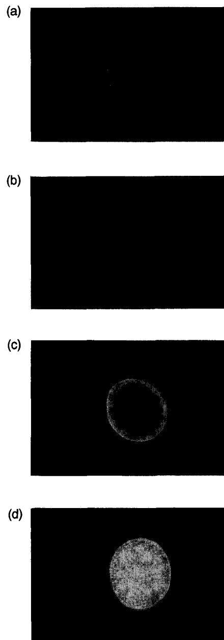
Fig. 8. Fluorescence microscopic photographs of cross sections of hair fiber into which a fluorescent dye, Sulforhodamine B, permeates from the hair surface for 60 min at 60 (a), 80 (b), 100 (c), and 120 °C (d).
